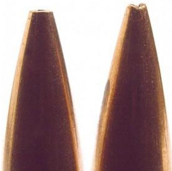
There will be variations in any box of hollowpoint match-style bullets, and a source for variation is the meplat (tip). Variations are an unavoidable result of the pointing-up process in manufacture. I've measured as much as 0.020 inches in a box. A "meplat
