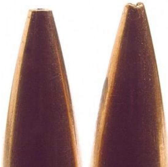
There will be variations in any box of hollowpoint match-style bullets, and a source for variation is the meplat (tip). Variations are an unavoidable result of the pointing-up process in manufacture. I've measured as much as 0.020 inches in a box. A "meplat uniformer" strives to eliminate this variance. Uniforming reduces the BC a scant few points, but it's a trade many serious long-range shooters say is worth the effort. Uniformed on left.
